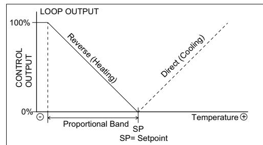
The temperature control loop can also be configured to operate as Proportional + Integral control by changing the Integral Action Time from 0 to a required value.
